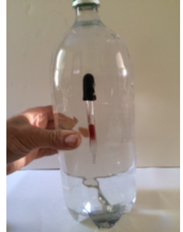
With just the right pressure the pipette is neutrally buoyant.
