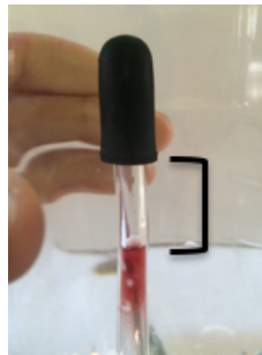
Air level in pipette when bottle is squeezed and pipette sinks.
