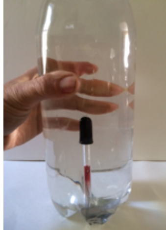
Squeezing the bottle sinks the pipette
