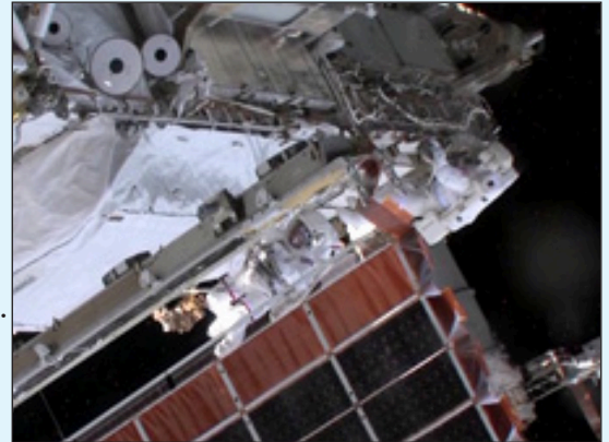
Flight Engineers remove a failed ammonia pump May 12, 2013. Photo credit: NASA TV
