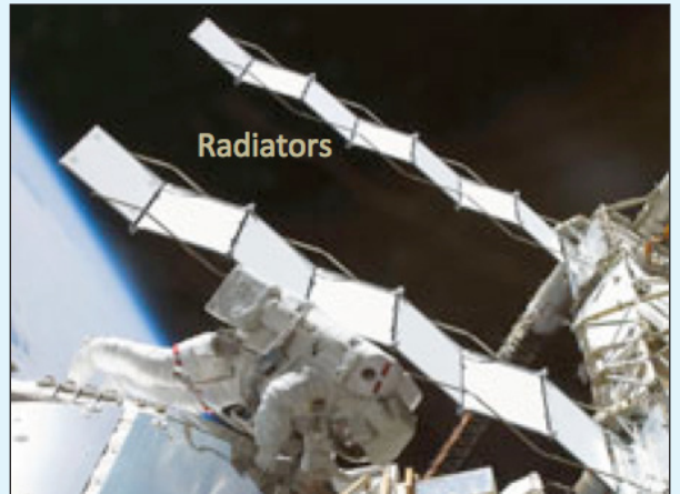
Pictured here are two of the many 6' x 12' radiators deployed from the ISS. Photo: NASA
